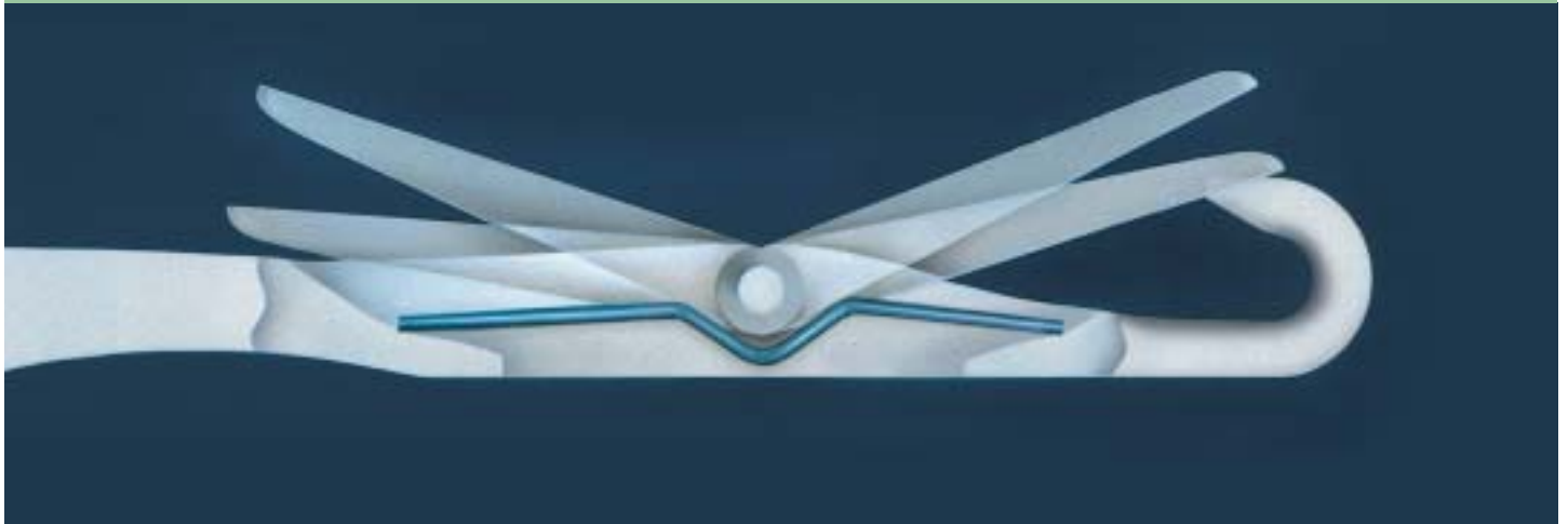
Sectional view – Spring loaded latch needle
