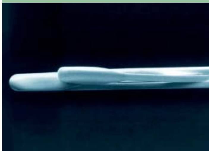
MAGNIFICATION OF A USED NEEDLE WITH BENT LATCH CAUSED BY CONTACT WITH THE YARN GUIDE
