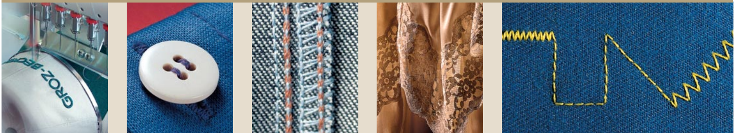
MULTI-HEAD EMBROIDERY BUTTON SEWING CHAIN STITCH FINE KNITWEAR BAR TACKING MULTI-DIRECTIONAL SEWING ZIGZAG
